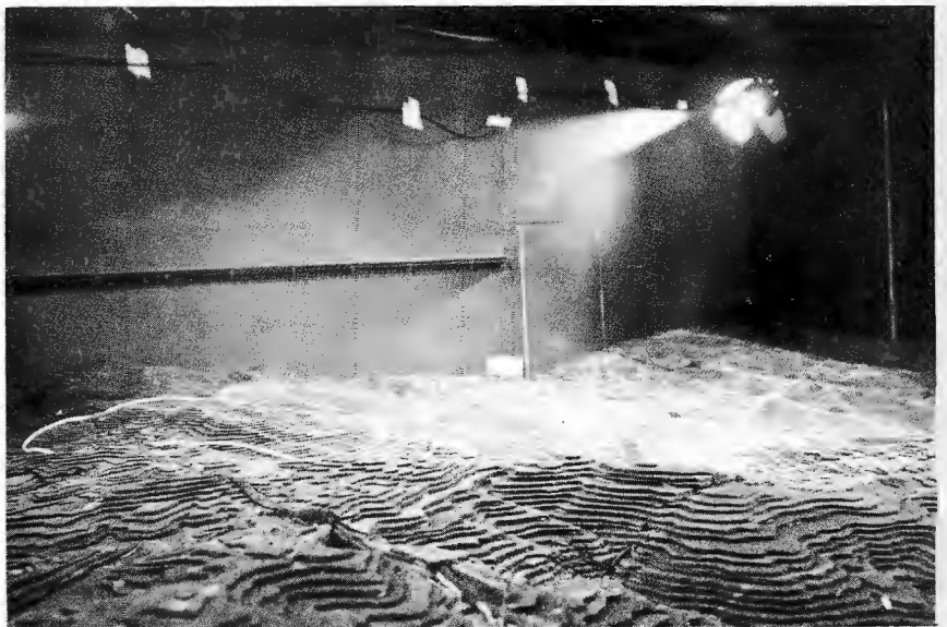
Figure 5.1-3 Stack release plume visualization for a 111.7 m/s exit velocity, 250° wind direction and wind speeds of a) 3.1 m/s, b) 6.2 m/s, and c) 9.4 m/s.
