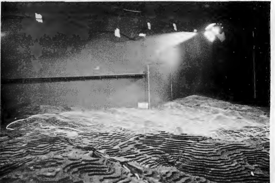
Figure 5.1-2 Stack release plume visualization for a 63.1 m/s exit velocity, 250° wind direction and wind speeds of a) 3.1 m/s, b) 6.2 m/s, and c) 9.4 m/s.
