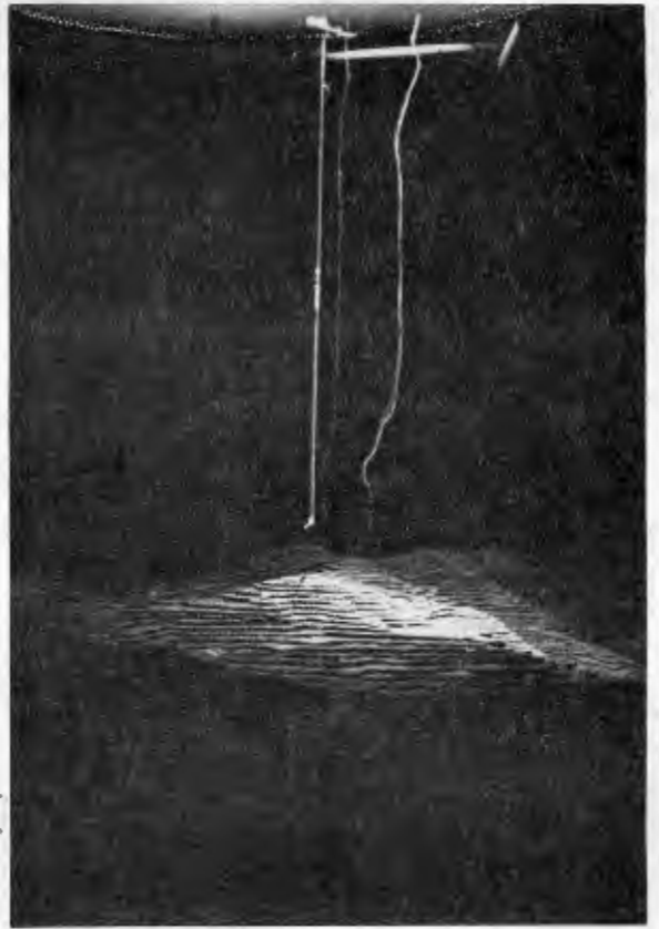
Figure 7.5 Smoke Wire Velocity Profiles (.05-second intervals) taken at three terrain heights in the Anderson Ridge Vicinity a) 975 m; b) 792 m; c) 719 m
