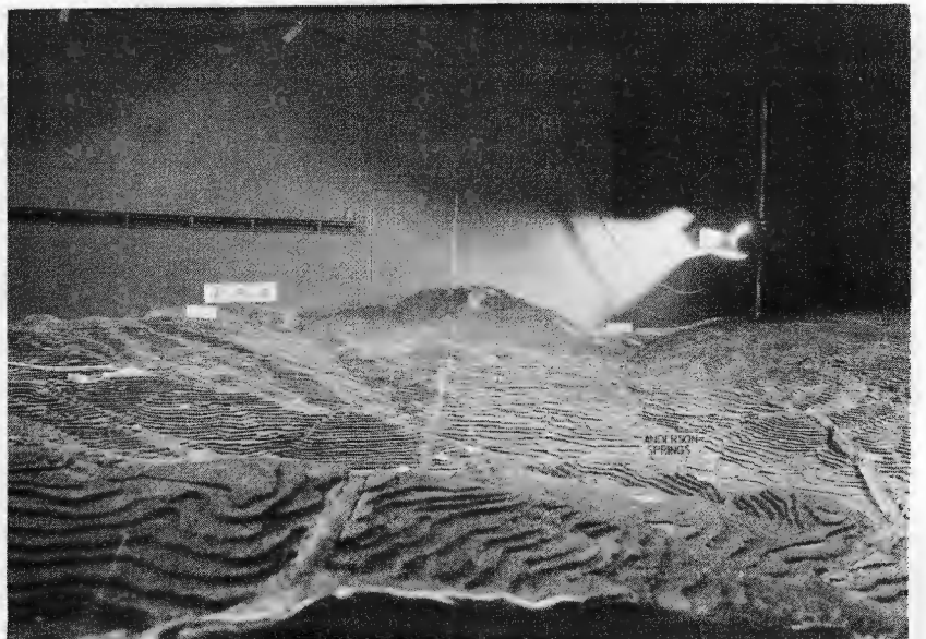
Figure 6.1-2 Surface stack release plume visualization for a 210^\circ wind direction, 9.4 m/s wind speed and exit velocities of a) 20.6 m/s, b) 63.1 m/s, and c) 111.7 m/s.
