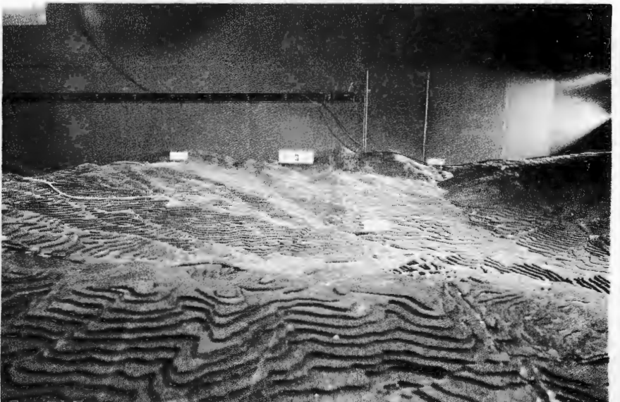
Figure 5.1-4 Stack release plume visualization for a 20.6 m/s exit velocity, 230° wind direction and wind speeds of a) 3.1 m/s, b) 6.2 m/s, and c) 9.4 m/s.
