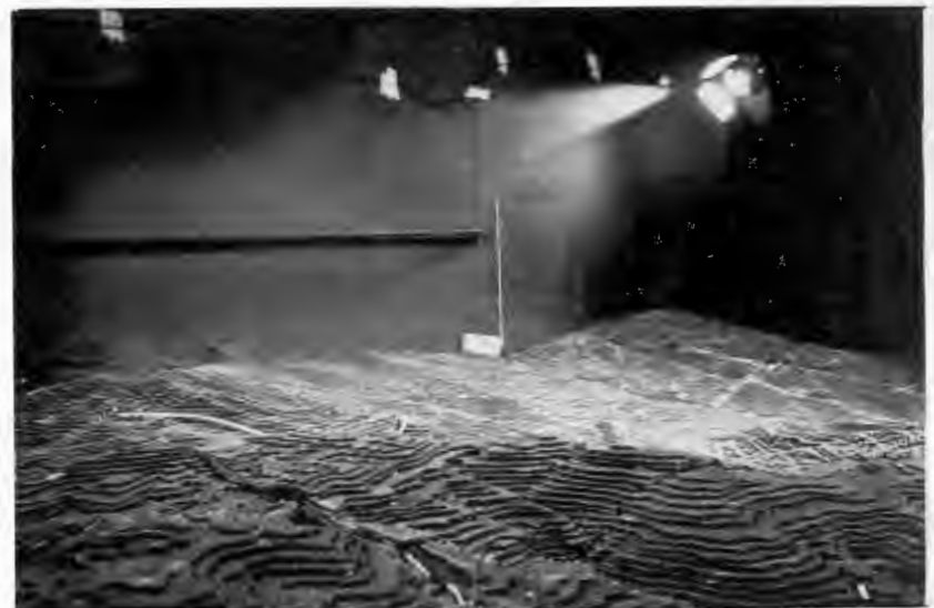
Figure 4.1-1 Surface release plume visualization for a 12.7 m/s exit velocity, 250° wind direction and wind speeds of a) 3.1 m/s, b) 6.2 m/s, and c) 9.4 m/s.
