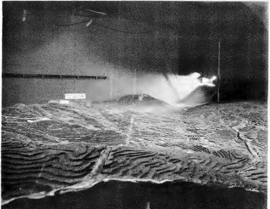
Figure 5.1-9 Stack release plume visualization for a 111.7 m/s exit velocity, 210° wind direction and wind speeds of a) 3.1 m/s and b) 6.2 m/s.
