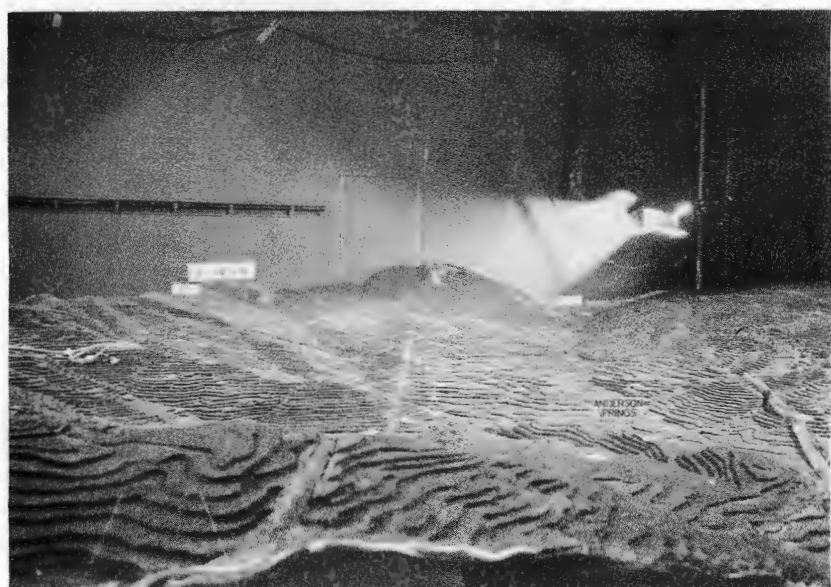
Figure 4.1-2 Surface release plume visualization for a 12.7 m/s exit velocity, 210° wind direction and wind speeds of a) 3.1 m/s, b) 6.2 m/s, and c) 9.4 m/s.
