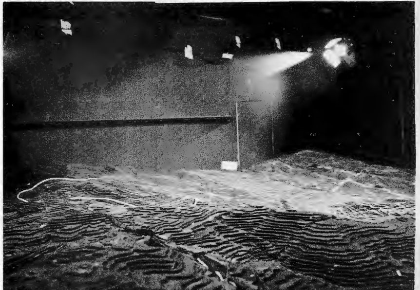
Figure 5.1-1 Stack release plume visualization for a 20.6 m/s exit velocity, 250° wind direction and wind speeds of a) 3.1 m/s, b) 6.2 m/s, and c) 9.4 m/s.
